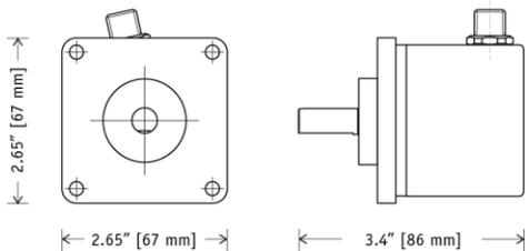
Introducing Celesco's CH25 Incremental Encoder. This encoder comes with a 2.5-inch square flange, 3/8-inch shaft and a push-pull output driver. The CH25 also accepts a wide input voltage from 5 to 30 VDC and is available in resolutions from 100 to 5000 pulses per revolution.
