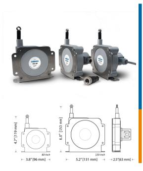
The SG1 provides absolute linear position up to a 10-ft. stroke range. Constructed with a rugged polycarbonate body, this model is available in an 80-inch or 120-inch stroke range and offers optional IP67 protection for wet or outdoor installations and an M12 connector for easy installation.
