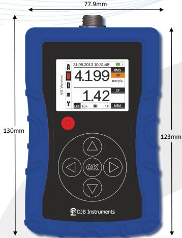
The VS1 is a compact, rechargeable, handheld Vibration Meter designed to conform to ISO10816-3 and operates with a constant current IEPE accelerometer providing accurate vibration measurement.
